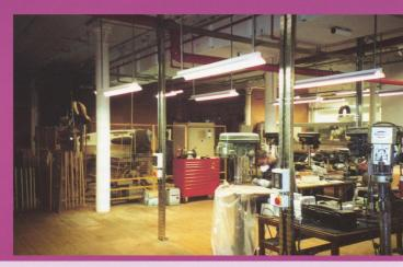
A versatile batten designed to meet the demands of heavy duty factory lighting or simple, unobtrusive cabinet and shelf lighting for retail. Using T5 lamp technology and the latest in low profile, high frequency ballasts the T5 batten offers energy efficiency combined with high output lighting. The combination of high frequency control gear and the T5 lamp offers a 20,000 hour lamp life, reducing maintenance costs.
